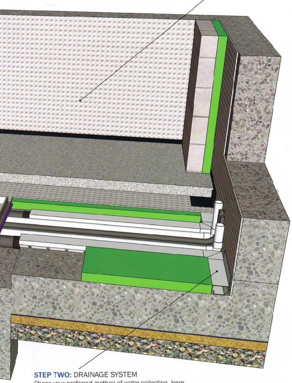
Chose your preferred method of water collection. Here Newton Basedrain is sat above the slab adjacent to a spacer of 50mm of closed cell insulation.
